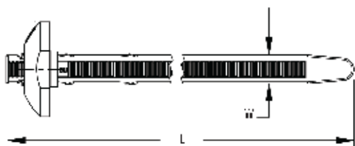
Fixing tie with deep hole anchor
