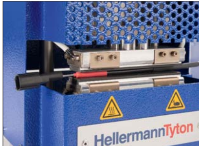
The foot switch initiates the shrink process. The two heated, special pads encapsulate the shrinkable product whilst transferring heat effectively with minimal heat loss.
