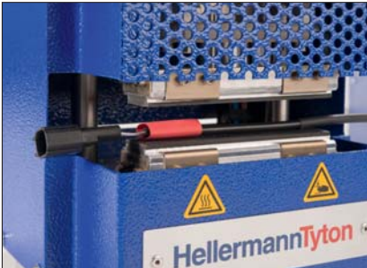
Put the object to be shrunk between the shrink pads.
