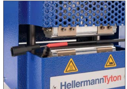
After the shrink time is over the shrink pads return to the original position. The shrink process has finished.
