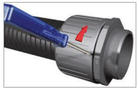
Move the handle of the screwdriver towards the "off" position. The capnut will rotate slightly. The locking mechanism is now released.
