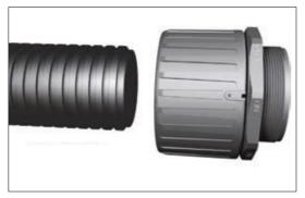
1. If the fitting has been used before, be sure that the slit points to the "on" position. To assemble the fitting, push it on to the end of the conduit as far as possible without forcing it and twist it slightly. The fitting is now securely locked.
