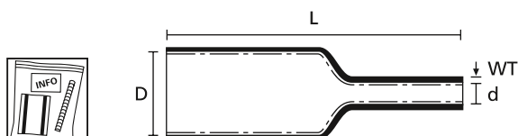
Heat Shrinkable Tubing 4:1 with adhesive
