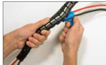
Simply slide the HAT applicator tool through the Helawrap cover.
