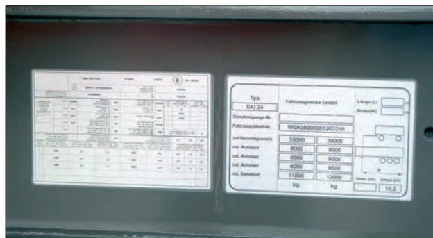
Type plate of an HGV trailer with protective laminate.
