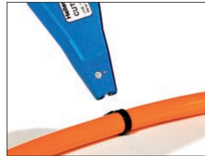
Bring the tool perpendicular to the tie...
