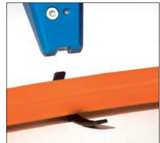
... release the button and remove the tool, the tie is cut.
