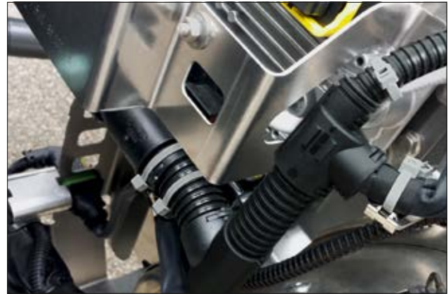
Application of PA46 cable ties at a truck exhaust unit.
