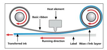
Heated dots strike a special colour ribbon, the thermal transfer film, which transfers liquefied colour ink at exactly that point onto the backing material (labels, tubes, rating plates). Our modern printers use what is known as "thin film technology", in which the very brief liquid phase of the ink produces faster print speeds and better and more precise images than with the "thick film technology" formerly used.
