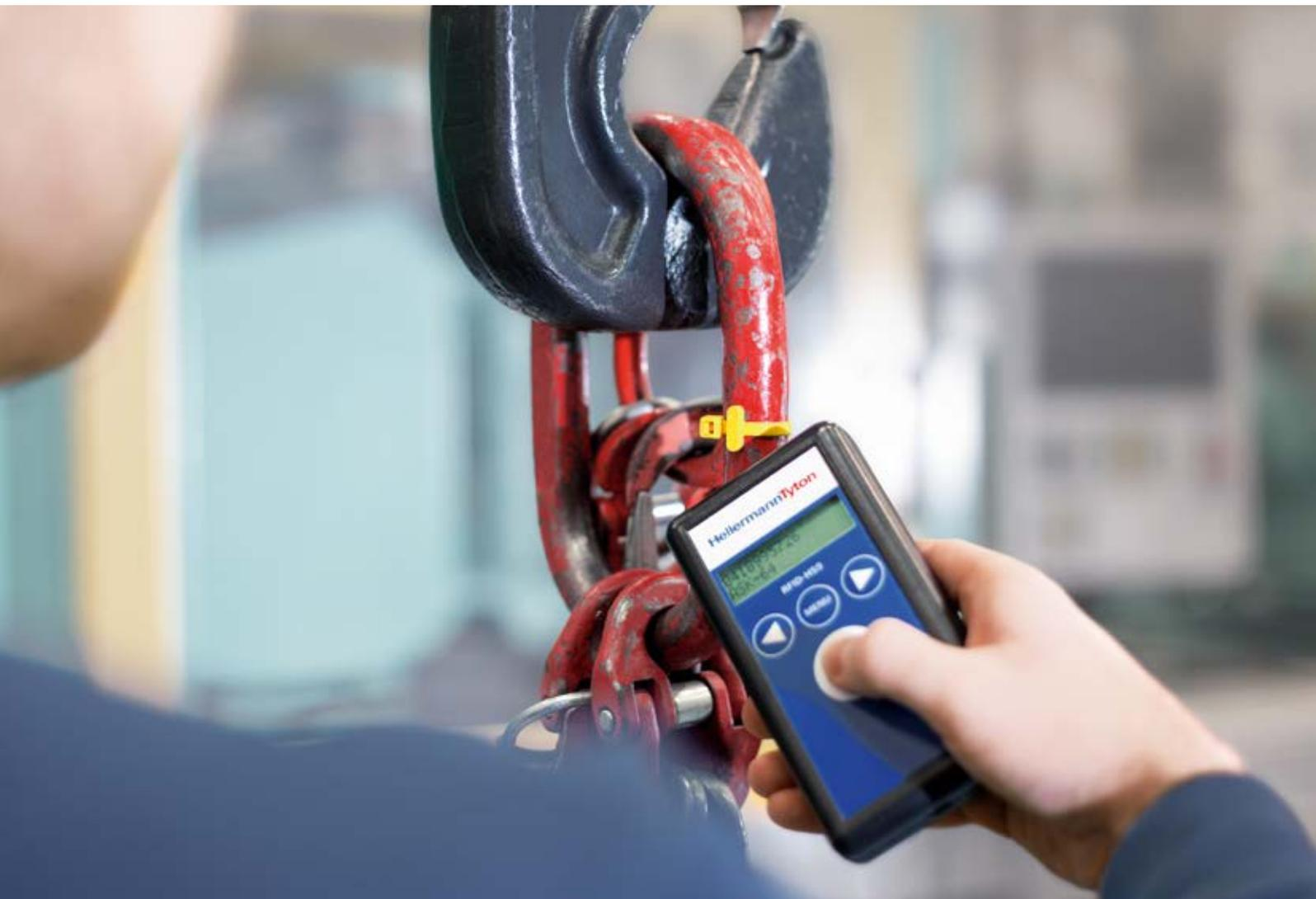
Three in one: information carrier, product label and fastener all in a single product! RFID technology, combined with the versatility of cable ties, provides highly flexible new opportunities for labelling and managing assets and tools with digital data.
