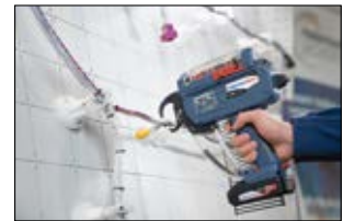
Battery-operated Autotool CPK hybrid applying cable ties from bandolier.
