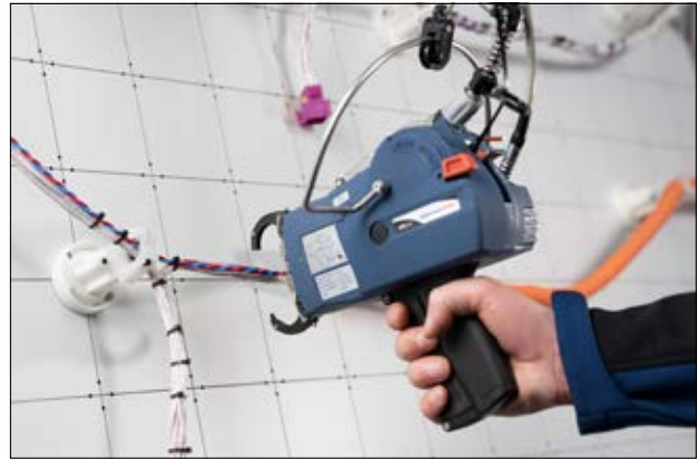
Autotool ATS flex on the harness board (also shown: Overhead suspension ATS).
