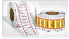
TULT DS is a UL-recognised 3:1 heat shrink marker. Made from polyolefin compound, TULT DS delivers good mechanical strength and resistance to organic solvents and chemicals. It is supplied in a convenient pre-cut "ladder" format suitable for double-sided printing.
