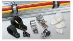
Conventional P-Clamps are ideal for permanent fixation of pipe and cable bundles. Aluminium withstands the most challenging environments. Chloroprene inserts counter vibration, reduce noise and provide electrical insulation. P-Clamps are also available in plastic material.
