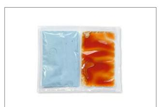
Two-component polyurethane cast resin PUR 33.
