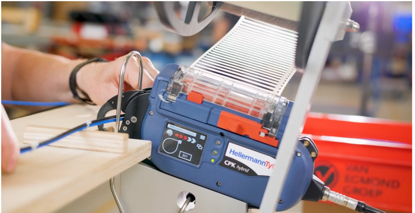
The CPK hybrid with Bench Mount Kit creates a dedicated workstation for high-frequency bundling tasks.
