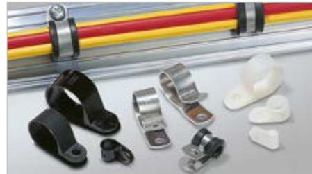
Conventional P-Clamps are ideal for permanent fixation of pipe and cable bundles. Aluminium withstands the most challenging environments. Chloroprene inserts counter vibration, reduce noise and provide electrical insulation. P-Clamps are also available in plastic material.
