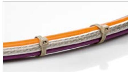
PEEK cable ties withstand temperatures from  $-55^{\circ}\text{C}$  up to  $+240^{\circ}\text{C}$ . They are resistant to gamma radiation and chemicals - even acids. The tie is outside-serrated and the head geometry optimised to minimise the risk of any damage to cable insulation.
