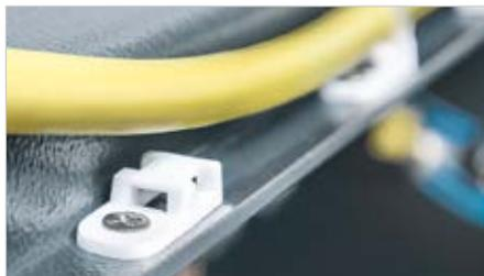
CTAM cable tie mounts are suitable for applications with minimal space. They are mounted onto equipment prior to cable installation. The CTAM has a 4-way entry design and can be used either in line or at 90 degrees to the cable run.
