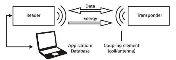
Radio Frequency Identification, for short RFID simply means the use of radio frequency waves to uniquely identify objects. RFID tags attached to items allow users to automatically and uniquely identify and track inventory and assets.
