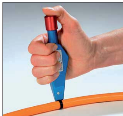
... press on the push rod by maintaining the pressure on the tool...
