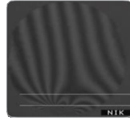
1,000 μm diameter fiber Interference microscope image 1 stripe = 0.01°
