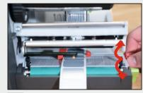
• Move and position the guides closely to the edges of the material by turning the knob (G) – do not squeeze the material
