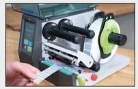
• Guide the consumable material strip underneath the internal winder towards the print head
