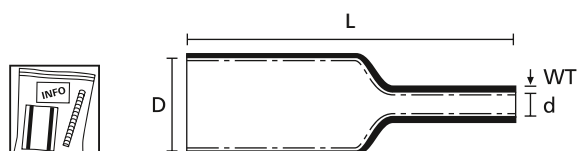
Heat Shrinkable Tubing 4:1 with adhesive
