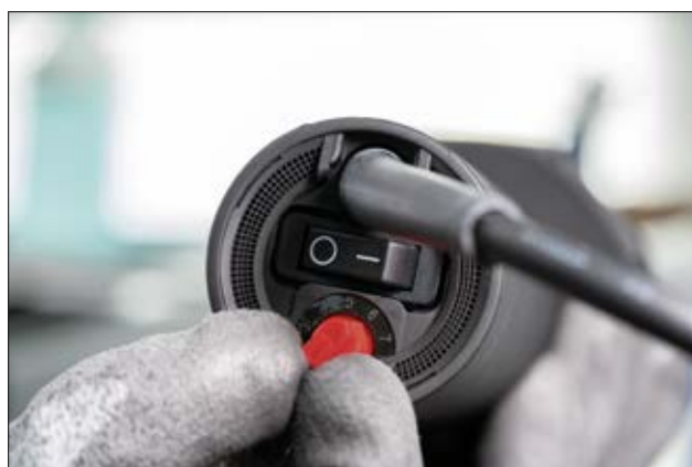
Adjusting H6100 operation temperature.
