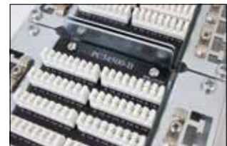
ZTB Internal view showing PCB trays with cable anchor points and shielding clamps
