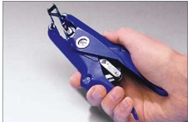
Fast, secure application with the three-pronged expansion tools.
