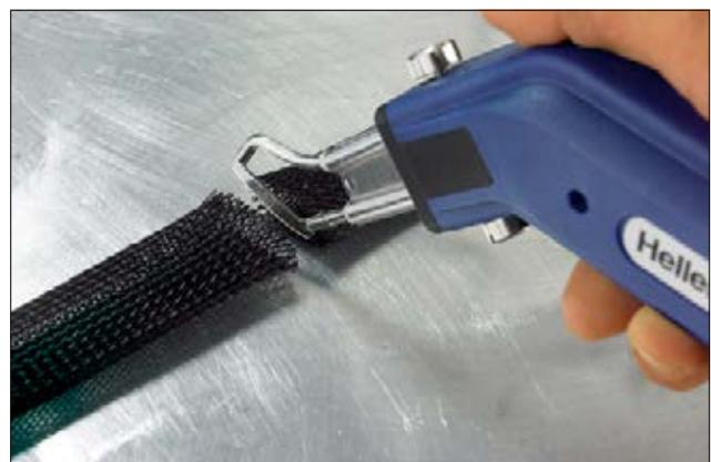
The HSGO hot cutting tool prevents the braided sleeving from fraying.
