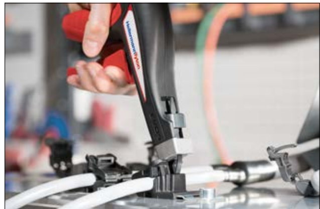
Tension tab can be used to ensure specific tension.
