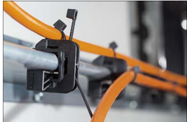
The Beam Clamp can be fixed onto a beam with a wedge. Up to two bundles can be routed on the top or rear side of the clamp.
