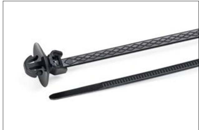
T30SOS-AS-SFT6.5x4E, 1 piece fixing tie with AntiSlip engraving for a round hole 6.5 mm or a square hole 6.5x4 mm.
