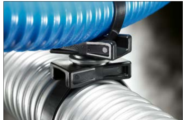
The spacers can be easily rotated by hand, allowing the bundles to be crossed and rotated at any angle.
