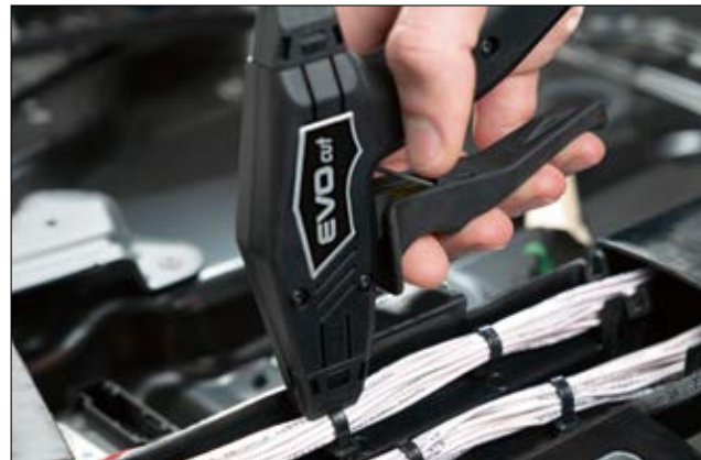
Tie can be cut off at any part of the strap.
