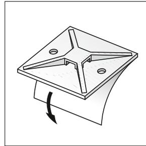
2. Peel off protective backing and ensure the adhesive area is not touched.
