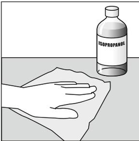
1. The surface must be dry, free from dust, oil, oxides, parting agents and other impurities. The surface to be glued should be cleaned using a clean cloth and isopropanol/water (50/50). When using other appropriate cleaning agents, ensure that they do not attack the surface nor leave any residues. After cleaning allow the surface to air-dry completely.
