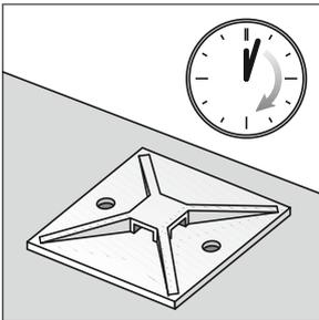
4. Depending on the type of adhesive, wait for several minutes (synthetic rubber) or hours (acrylate) so that the adhesive can bond completely with the surface.
