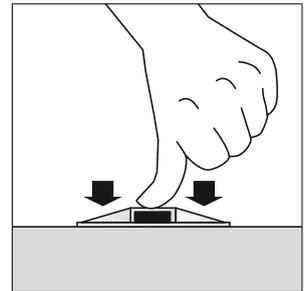
3. Press down firmly on the base with the thumbs for several seconds.
