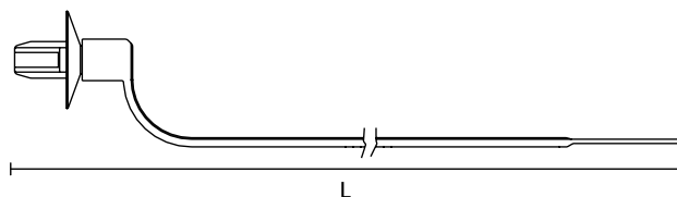
Special design without a gap between head and bundle; T50MD7
